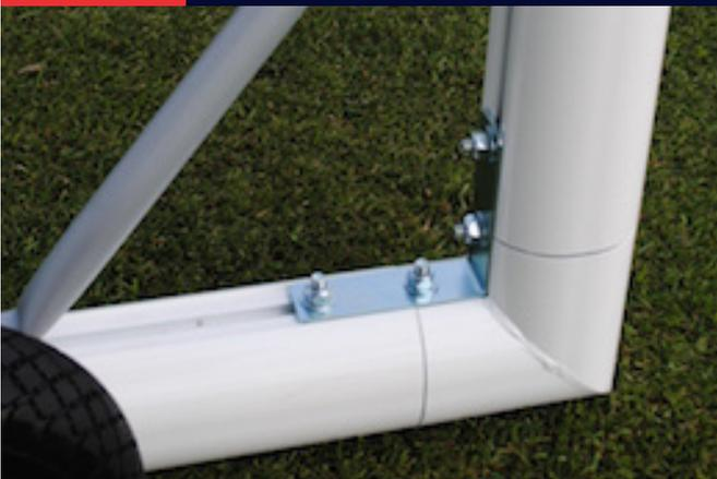
Aluminium that has been simply cut or mitred tends to separate, leaving sharp exposed corners. It's important if you have this type of goal to regularly check they are still safe to use, as they can cause serious injuries. Goals with welded corners don't have this issue as a smooth weld covers the edge; however it is still important to check these as misuse or old age can cause the aluminium to crack.
